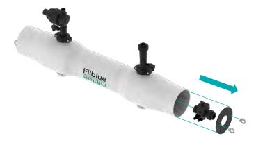
You can then unscrew the screws that hold the retaining ring in place and remove them from the filter body **Filblue FBL2000A**:
